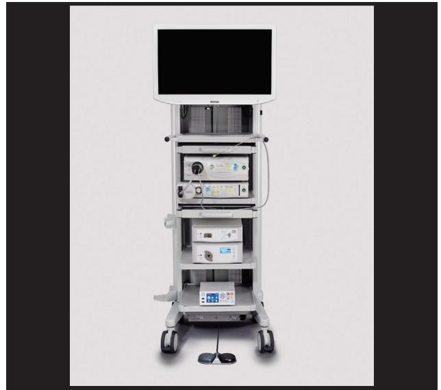
automatic gain control (AGC) and dynamic contrast function. In addition, selective color enhancement, smoke reduction and grid removal features all enhance observation abilities. A High Power 200 LED Light Source allows the user to adjust the intensity of the light from 5-100%—providing operational efficiency and lowering power consumption.
